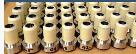
M-24231 Plug Sleeves Coated with NCC 209™
